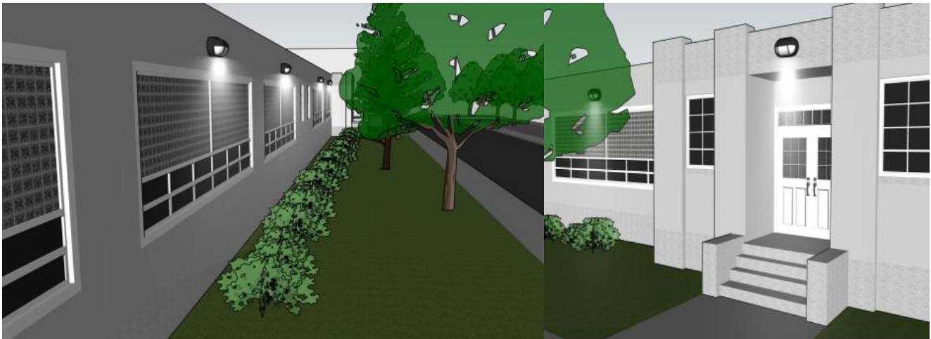
Figure 11. Lighting on the Exterior Wall and Over the Building Entrance
